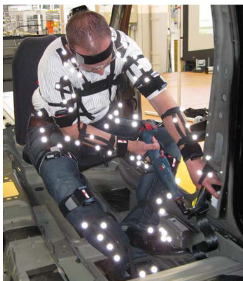
Fig. 2: Example of an assembly operation with Hybrid Motion Capturing with optical targets and inertial sensors
